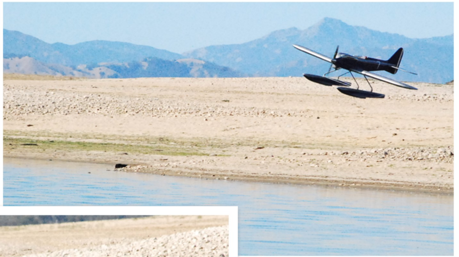
RICH'S SUPERMARINE SCHNEIDER CUP RACER; SCRATCH BUILT FROM PLANS SCALED UP FROM A SMALLER VERSION
